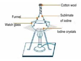
Figure 5.17: Sublimation apparatus setup
