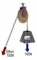
Figure 9.4(b): A fixed pulley
