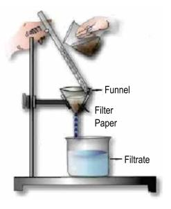
Figure 5.13: Filtration apparatus setup
