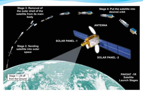
Figure 12.10: Launching of PAKSAT-1R satellite into space
