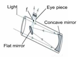
Figure 10.15: Amirror is used for the reflection of light in to the reflecting telescope. It is used to examine the visible light.
