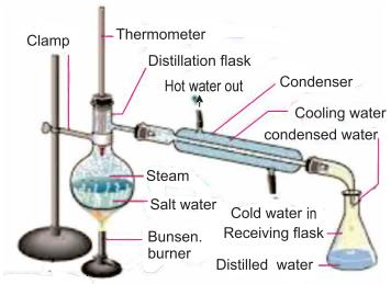
Figure 5.16: Distillation apparatus setup
