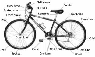
Figure 9.14(a): Parts of a bicycle
