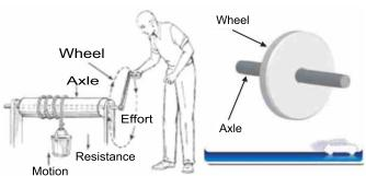
Figure 9.2: Various wheel and axles
