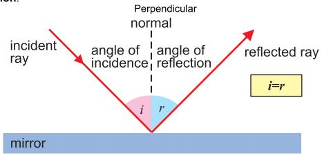
Figure 10.6: Light wave being reflected
