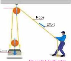
Figure 9.6: A double pulley
